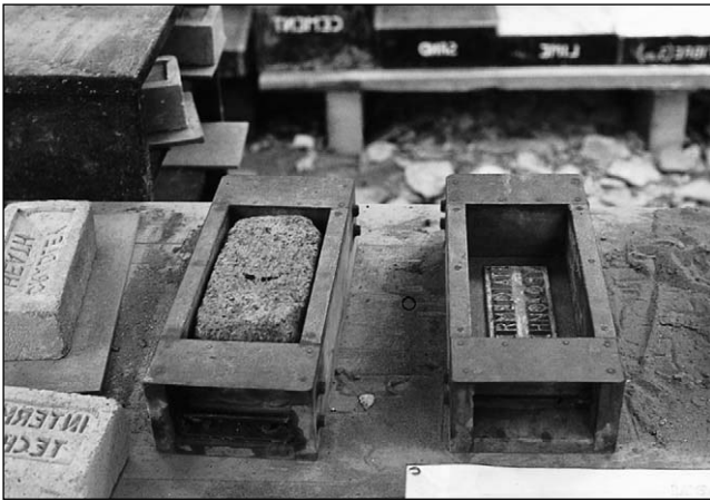
Figure 8.8: Wooden mould for handmade bricks.
